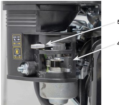
6. Put engine switch to the **ON** position. It will be a switch on the side of the engine as shown below.
