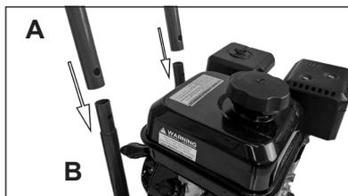
2. Insert the bolts through the holes. The bolts will have hex heads that need to be matched to the sides of the handles with a hex-shaped hole pattern to help secure them. Thread on the plastic fasteners and tighten by hand.
