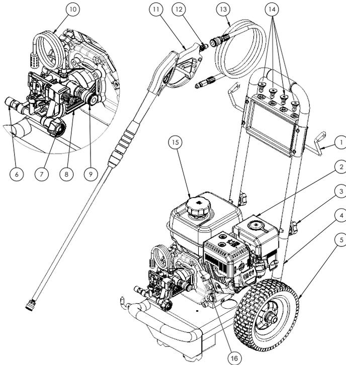
1. Frame hook: Storage for the pressure washer hose or spray gun wand.
