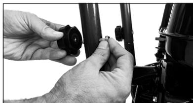
3. Insert colored quick-connect spray nozzles, high-pressure hose, and gun wand assembly into the spaces provided.
